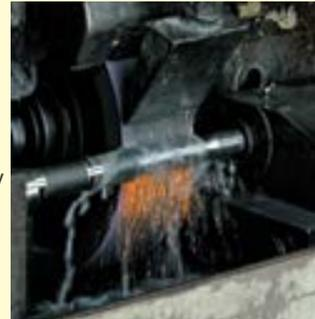
Centerless Grinding Wheels
